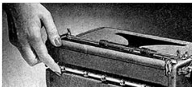
Setting the tab stops on the Royal Portable Quiet De Luxe.
