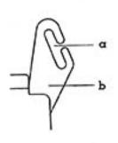
shift lock, and take hold of the ribbon with both hands. Put the ribbon behind guide (b) and insert it into the left and right slits of the guide (a) so that its full width lies in the slits. When correctly fitted the position of the ribbon will correspond to that shown in the diagram
