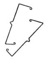
Remove the wire springs from the left and right of the carriage. To do this turn the machine on its back and press out the wires from under the sides, lifting them up in the direction of the carriage and shaking free.
